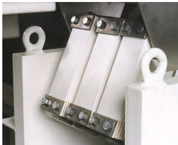
Fiberglass springs attach the base to the trough and enable tuning of the conveyor
