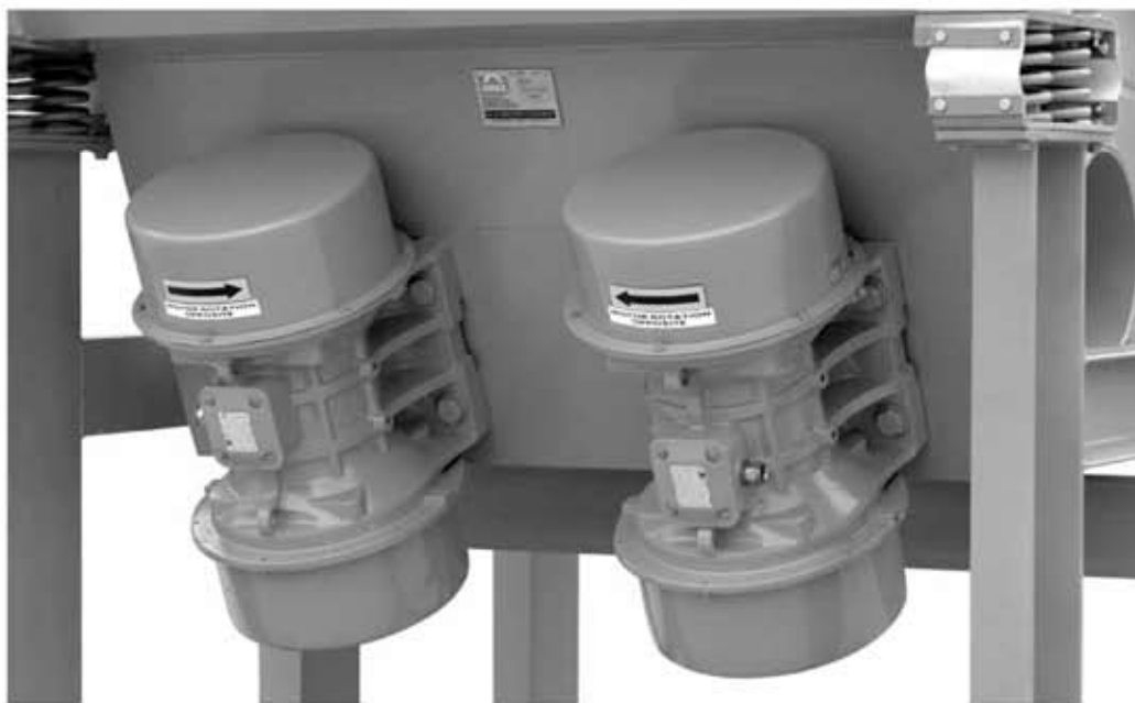
Counter rotating rotary motors provide the driving force and stability required for heavy duty applications.
