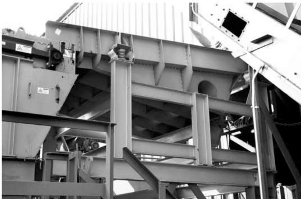
Eriez Brute Force feeder distributing material onto a belt in a scrap sorting application.
