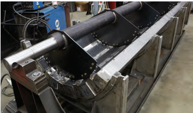
Construction of a wet drum magnet element
