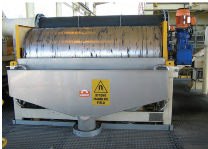
Model CDA Wet Drum Undergoing “In-Plant” Testing
