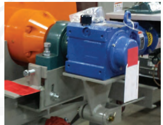
Direct Drive - Shaft Mounted Gearmotor
