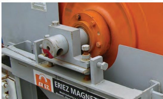
Self-Leveling Counter-Rotation Tank - Drum Positioning and Magnet Adjustment
