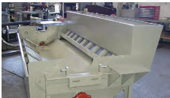
Self-Leveling Counter-Rotation Tank
