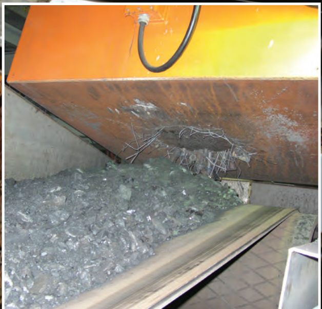
These images are two examples of manual-clean magnets pulling unwanted metals out of conveyed products.
