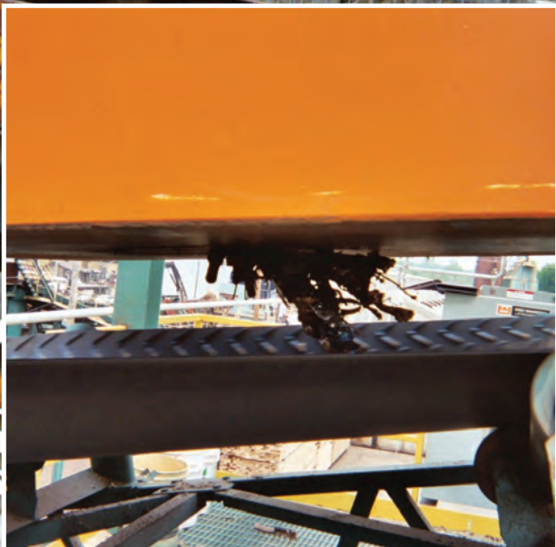
Suspended magnets play an important role removing dangerous tramp or rogue metal from conveyed materials.
