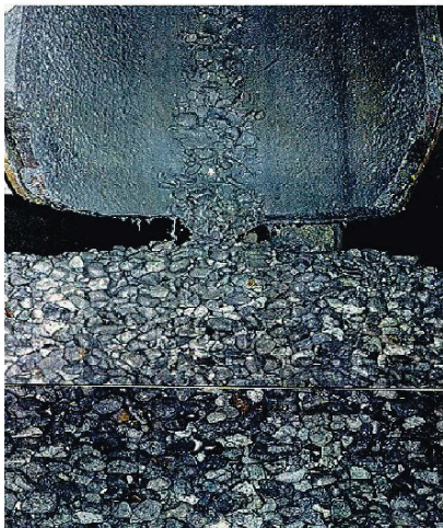
Grinding ball chips collected by the Trunnion Magnet System.
